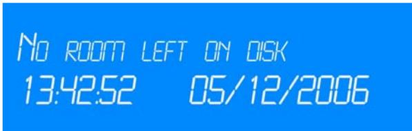
A: Press "Stop" to clear this message. It will be necessary to upload and delete some files from your 73fifty before further recording is possible. Note that the deletion process is not complete until the 73fifty has been power-cycled.
