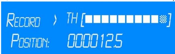
A: This message is a warning that disk space is becoming full. The more chequered boxes that are displayed, the less space there is left on the disk. When you see this message it will be necessary to upload some files (for example to a Windows PC). If this is not done, eventually the disk will become full and recording will no longer be possible until some files are uploaded.
