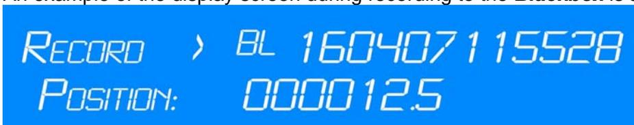
The first line of display indicates that the unit is currently recording. The BL indicates that it is a **Blackbox** and is recording at low bitrate. The line of digits shows the current file name (the date and time the current recording segment began.)
