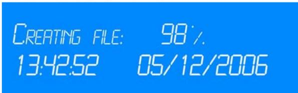
A: This is a feature of recording in time-restricted mode. The message means that more than 5 minutes of data has been recorded and a 5-minute segment is being created. Please be reassured that recording is still in progress. After a few seconds this message will disappear and the screen will say "Record" again.
