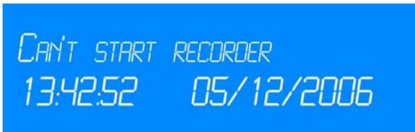
A: This message is displayed when "Record" is pressed but the disk space is already full. The "Can't start recorder" message alternates with "No room left on disk". Pressing "Stop" clears the message. It will be necessary to upload and delete some files from your **73fifty** before further recording is possible. Note that the deletion process is not complete until the 73fifty has been switched off and back on again.
