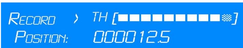
The more boxes that are chequered, the less space there is. Note that the unit is still recording at this stage. However, you should upload some files to a Windows PC as soon as possible.
