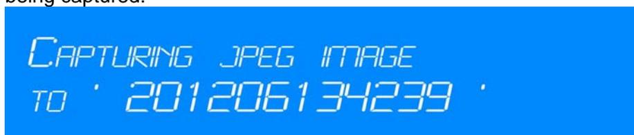
The second line of the display indicates the filename being given to the stills grab. Please note that the **filename** of the stills grab will be the date and time **when the grab was taken** (not when the file was originally recorded).
