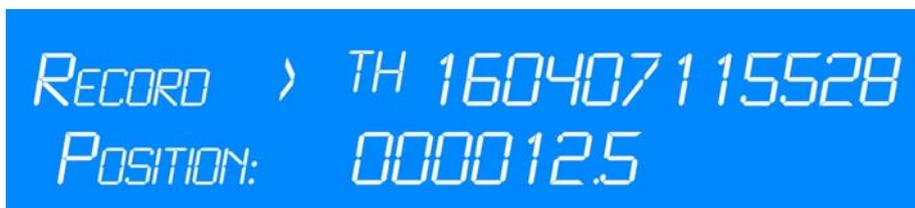
The first letter indicates whether you are recording in continuous (c ) or time-restricted ( t ) mode. The second letter indicates whether you are recording at high (h), medium (m) or low (l) bitrate. In the above example the **73fifty** is recording in time-restricted mode, at high bitrate.
