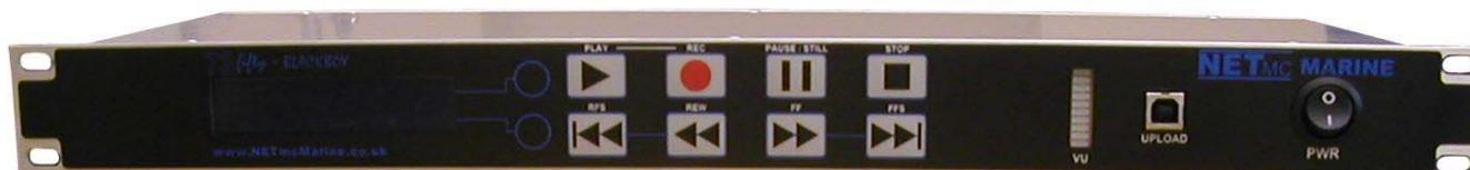
The **73iftyBlackbox** is designed for recording for HSE purposes. The unit records to an internal hard disk. Files can be uploaded on to a Windows PC in the same manner as for the standard (blue) **73ifty**. Once the disk is full (after 44 to 83 hours dependent upon the bitrate selected) the unit loops automatically – i.e. the earliest files recorded are deleted to make way for the new ones.
