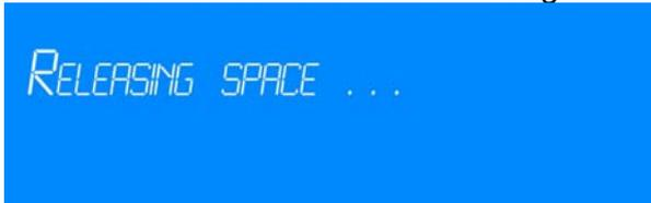
A: This is a feature of the loop-recording of the **73iftyBlackbox**. Once the disk space has been used up, the unit will start progressively removing the oldest files to make room for the new one. You will see this message every 300 seconds. Recording is not interrupted whilst this message is displayed, and it is not possible to stop recording until this task has been completed.
