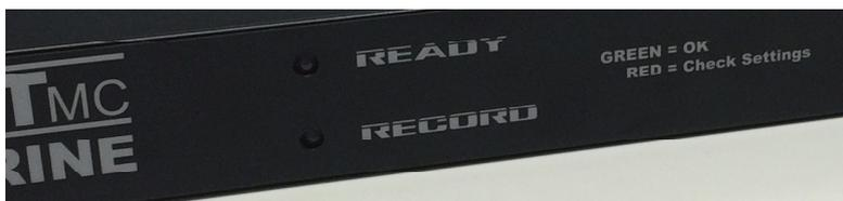
Two indicators are provided on the front panel to give the user confidence that the unit is functioning.
