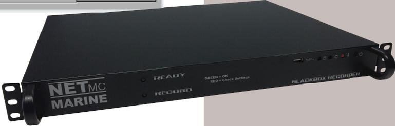
New in this model is the option for a built-in video overlay module, this allows the Black Box to be a complete separate entity from the rest of the video suite. The format has changed from MPEG2 to the more ubiquitous MPEG4 but of course we have kept the popular 12V trigger and 1U 19" rack format.
