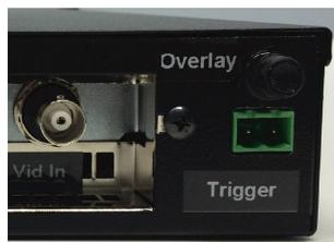
When 12v is supplied to the rear connector, recording will start and will only be stopped by removing the 12 input (software application controls will be disabled).
