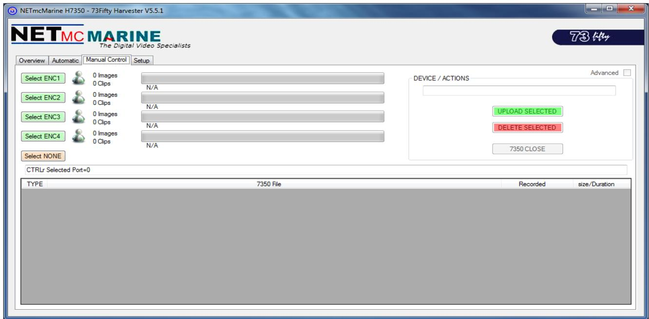
The user should click on the Channel relating to the particular recorder to be searched (selected channels change colour) – then a list of files will be shown.
