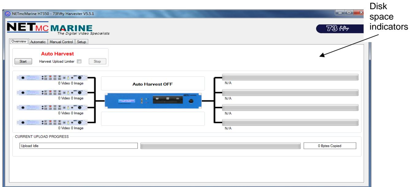
The disk space indicators indicate the space available in the target storage drive being used for the upload of files. As each **73fifty** recorder can save to a different location, each drive is shown separately.
