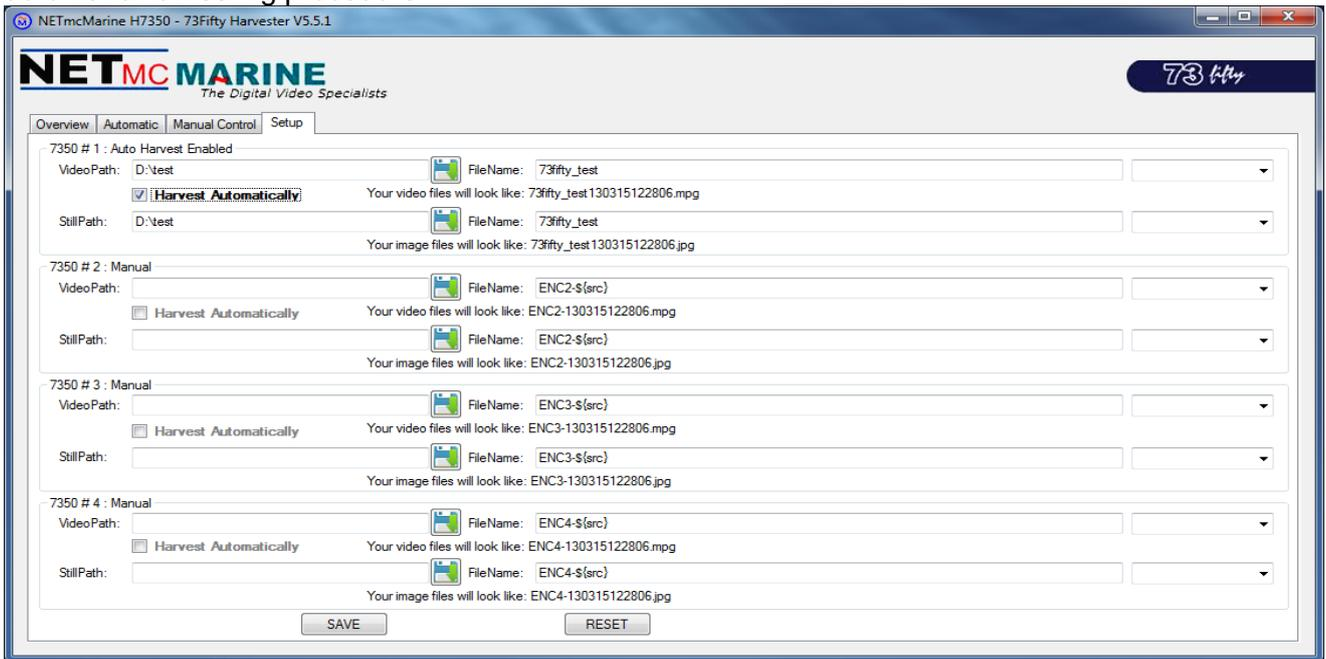
The **73fifty Harvester PC** will begin to upload files from the selected recorders immediately regardless of whether the **73fifty** recorders are currently recording or idle. Any recording in progress will not be interrupted.
