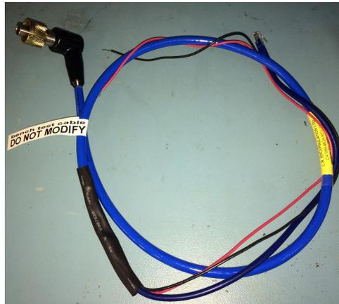
This is a short cable to link the camera directly to the topside unit and allows the connection of 24v (from a bench supply) to power the camera. This should be preserved for testing and another cable used for the underwater splice into the vehicle. (additional cable can be ordered from NETmc Marine)
